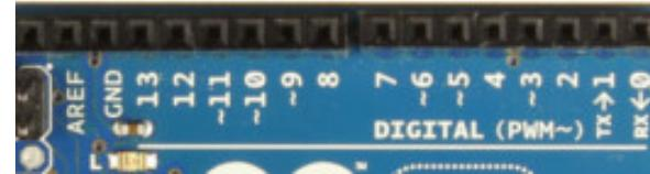
Finally, connect the Arduino digital output pins to the driver module. In our example we have two DC motors, so digital pins D9, D8, D7 and D6 will be connected to pins IN1, IN2, IN3 and IN4 respectively. Then connect D10 to module pin 7 (remove the jumper first) and D5 to module pin 12 (again, remove the jumper).
