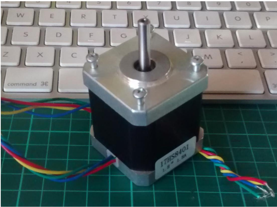
It has 200 steps per revolution, and can operate at 60 RPM. If you don't already have the step and speed value for your motor, find out now and you will need it for the sketch.
